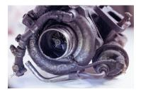
Replace the oil feed pipe, as it's crucial for proper turbo lubrication. Don't rely on simply blowing through pipes to test them; internal cracks can obstruct oil flow. Clean or replace the oil return hose to prevent flow restrictions. Install new oil, air, and fuel filters, addressing any excessive soot or sludge before proceeding. Fill the new oil filter with fresh engine oil if possible for immediate lubrication upon start-up.
